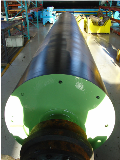
Figure 10. DuraTrax™ Covered Roll With Sealed Heads.
