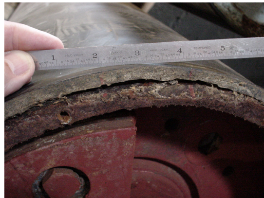
Figure 9. Edge-Lifting In a Rubber Covered Roll
